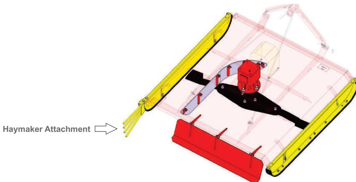
Note: Always use Winged Blades with the Haymaker Kit and always use Standard (Tilted) Blades for Normal Operations. And ensure that the Winged Blades is the correct way around. The 'Wing' side of the blade must face upwards and follow the cutting edge when rotating.
